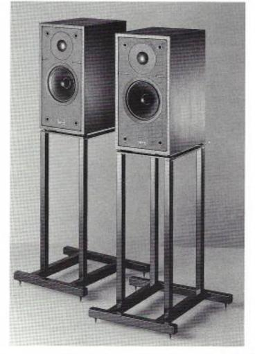
dome treble unit is designed for this system, providing an extended downward frequency range. Extension is aided by a bored pole and rear cavity, with control exercised by ferrofluid in the gap. Bar a 15 ohm resistor across the HF voice-coil, the sole crossover component is a 1.5μF polypropylene capacitor to the tweeter. The bass-mid is direct-coupled to the amplifier, and sounds it. Its upper frequency range is augmented by a fixed phasecorrecting nose-cone mounted on the pole face.
